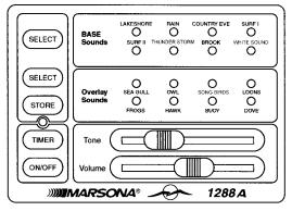
remain on. To move on to other overlay selections, touch the select button twice. With the first touch, the lamp will begin flashing; touch select again to move on to the next overlay. To store or save additional overlays, repeat the process of touching the store button for those overlay sounds you wish to save.
